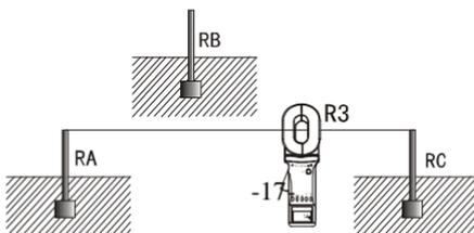
In the above three steps, the reading measured in each step is the value of the two series grounding resistance. In this way, we can easily calculate the value of each grounding resistance:
