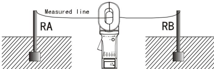
As the resistance value measured by the Meter is the value of the series resistance from the testing line and two grounding resistances.
