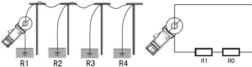
Where:  $R_1$  is the target grounding resistance.
