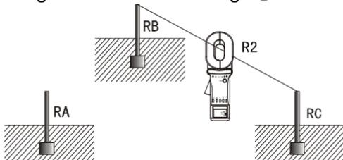
Third, have  $R_C$  and  $R_A$  linked up, as shown in the following figure. Use the Meter to get the third reading  $R_3$ .
