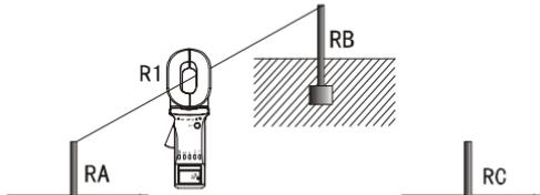
Second, have  $R_B$  and  $R_C$  linked up, as shown in the following figure. Use the Meter to get the second reading  $R_2$ .
